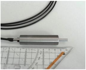
Fig. 20 Weight attached to the dipping probe
