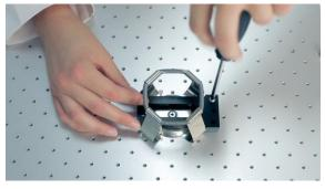
Fig. 7 Fastening the CFG guide rail to the shaker tray with a screw
