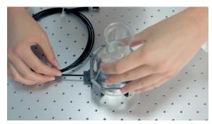
Fig. 10 Positioning the optical module and the sensor integrated in a shake flask
