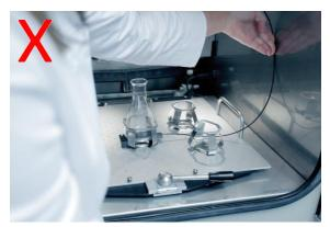
Fig. 12 Wrong positioning of the polymer optical fiber; it will beat against other parts during shaking movements
