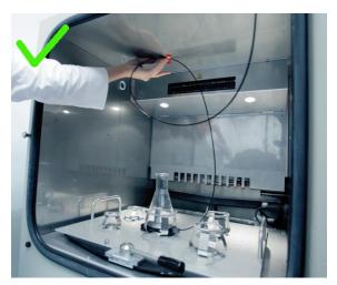
Fig. 13 Right positioning of the polymer optical fiber; adhesive tape is used to hold it in place
