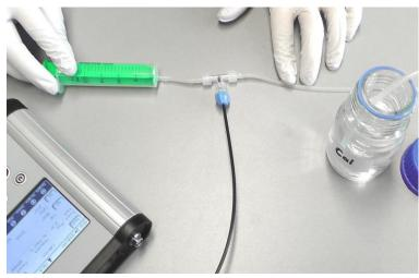
**Fig. 8** Calibration set-up: The FTC-SU-PSt3 is connected with tubing to a container with calibration solution and to a syringe.
