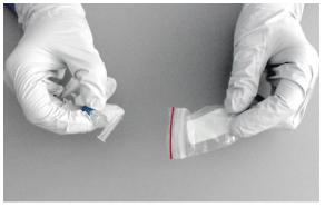
Fig. 5 FTC-SU-PSt3: the sensor stick is attached to a disposable T-cell.
