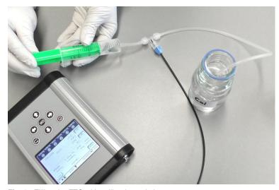
Fig. 9 Filling the FTC with calibration solution
