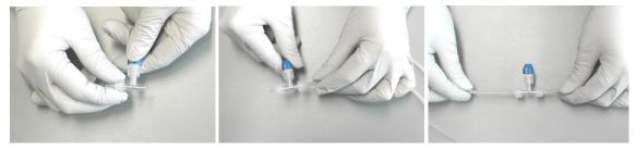
Fig. 6 Connecting the FTC with the tubes of the perfusion system (using Luer-Lock adapter).
