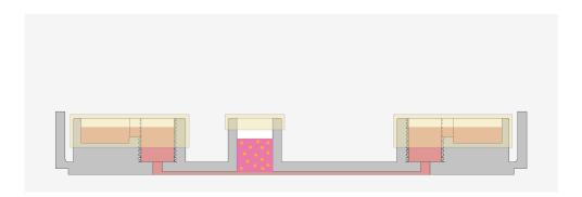
**Important:** Do not remove the medium inside the channel during medium refreshing. This will prevent the entrance of air bubbles. Thus, when removing the solution, place the tip of the pipette away from the pinhole to avoid emptying the channel.
