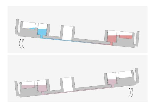
**3. Aspirate** the dilution buffer/coating solution <u>completely</u> before seeding.
