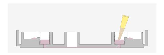
**Tip**: a 1 mL tip may help in a more efficient aspiration by the two inlets several times.
