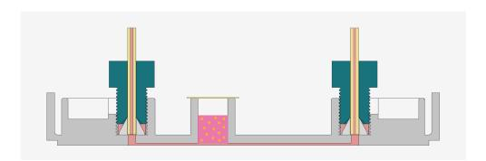
**Check** that there are no leaks in the system by leaving the pump running for a couple of minutes before placing the device in the incubator. Medium reservoirs will be filled up if the connections are not completely closed.
