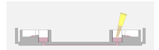
**Important**: Note that the channels should never dry up. Take incubation times into account and use the evaporation reservoirs as long as possible.
