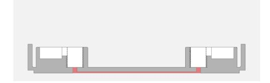
Note: Another way to proceed is to **pipette the solution into the inlet well** and **let the liquid flow** by itself through the channel **until it reaches the outlet well**.
