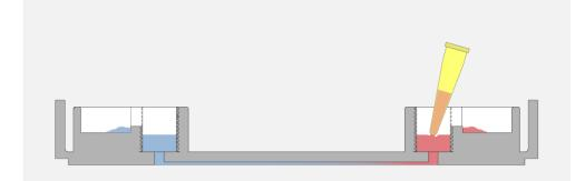
**Tip:** You may **tilt the device** manually in order to ease the dilution buffer flow **several times** from one reservoir to another before you remove it.
