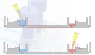
Important: Note that the channel should never dry up. Take incubation times into account and use the evaporation reservoirs as long as possible.
