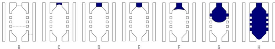
2. In order to confine the chip it must be completely dry inside the chamber (B).
